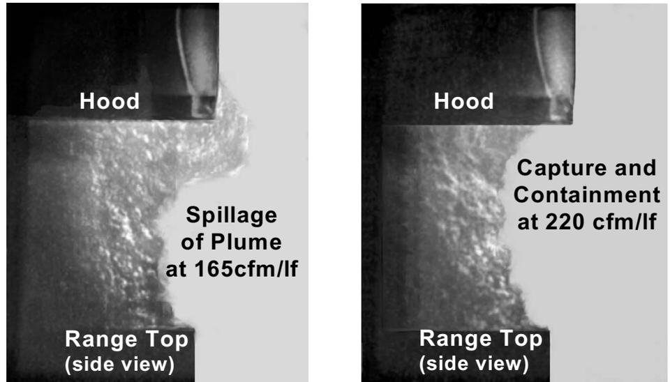
**Figure 2. Schlieren images at different exhaust rates per linear foot (lf).**
