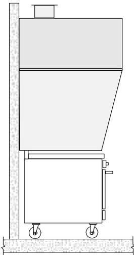
**Figure 12. Illustration of partial and full side panels.**
