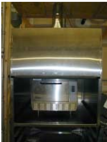
Figure ES-1. TurboChef C3 inside test hood.
